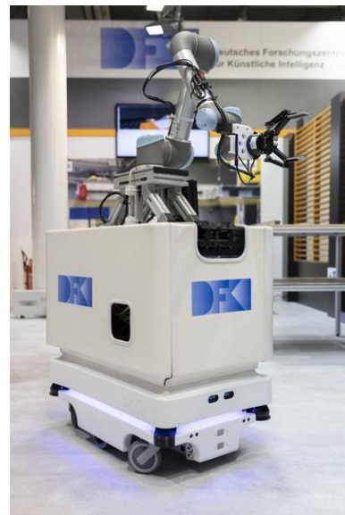
Figure 1: The Mobipick custom robotic mobile manipulator, consisting of a MiR base, UR5 arm and Robotiq gripper.
