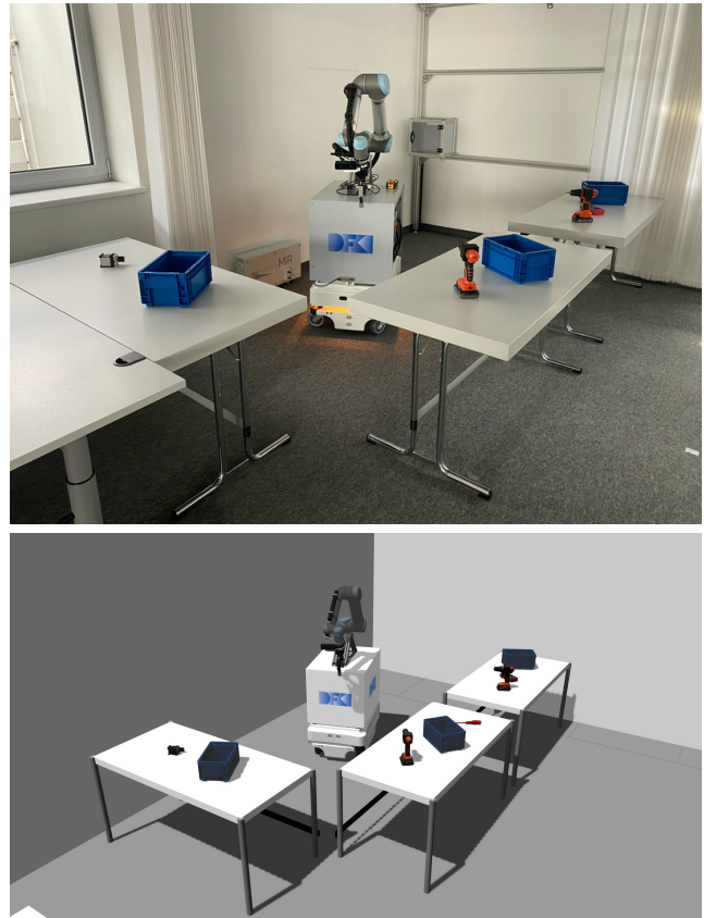
Figure 3: Example of one of the provided pick and place environments. Top: real environment, bottom: simulated environment in Gazebo.
