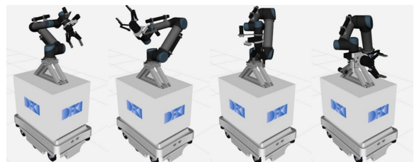
Figure 7: Some pre-recorded named arm configurations: home, observe100cm_right, transport, handover; e.g., transport = [-0.89, -1.87, 2.13, -1.82, -1.57, 3.80]
