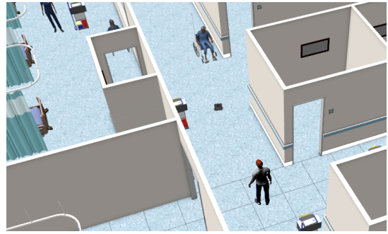
Figure 7: Snapshot of the simulation. One person is in a wheelchair in front of the robot and another behind. PTDRL selects parameters that are aware of the crowded situation.
