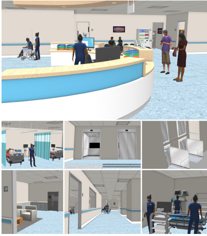
Figure 2: A simulated hospital (AWS RoboMaker 2021) with humans walking according to social forces (Helbing and Molnár 1995), and a robot travelling through rooms. Collision avoidance, safety and fast movement is needed for the robot to be deemed useful in such an environment.
