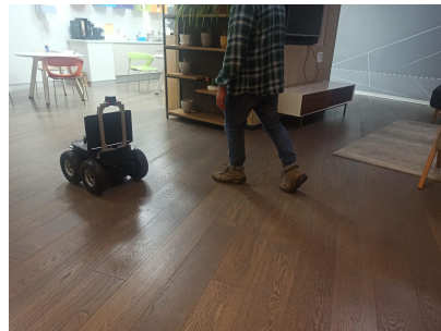
Figure 1: A robot navigates autonomously among people. According to sensor readings it is able to adapt navigation system parameters to have more desired behaviors.
