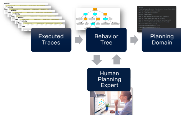
Figure 1: The proposed approach generates planning models from a set of execution traces using Behavior Trees as an intermediate representation in order to engage human planning experts and account for their experiential knowledge.
