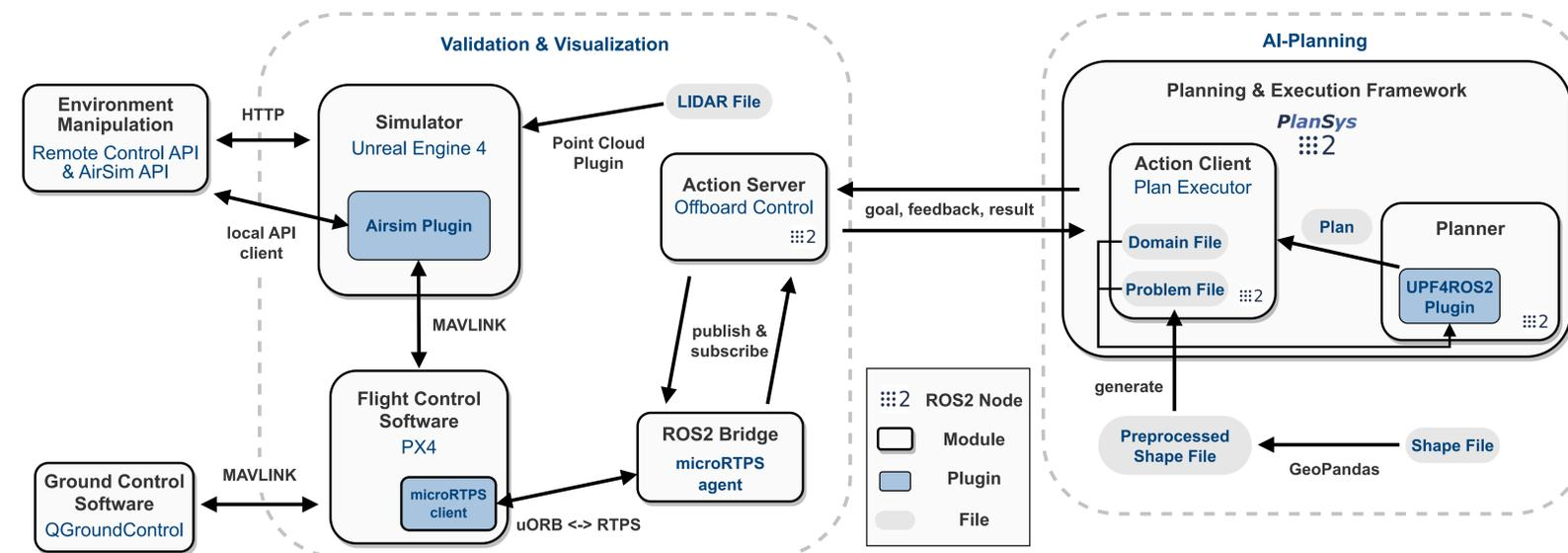
**REAP** is a simulation framework for Unmanned Aerial Vehicles (UAVs) that integrates state-of-the-art AI-planning tools into a visually realistic environment using open-access real-world data.
